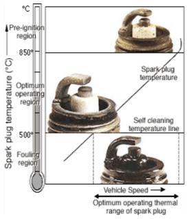
The firing end appearance also depends on the spark plug tip temperature. There are three basic diagnostic criteria for spark plugs: good, fouled and overheated. The borderline between the fouling and optimum operating regions ( $500^{\circ}$ C) is called the spark plug self-cleaning temperature. The temperature at this point is where the accumulated carbon and combustion deposits are burned off.
