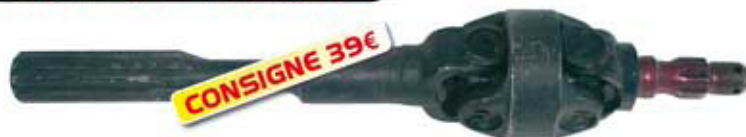
Cardan roue double croisillon (long. 470mm, 8 cannelures) 3002013 Consulter : 2cvclub.com
