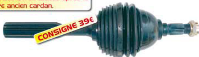
Cardan roue double croisillons (long. 396mm, 22 cannelures) 3002015 Consulter : 2cvclub.com
